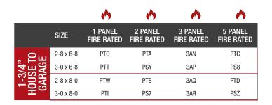
**Note:** 8-0 doors in the 5 Panel series will have 6 panels **Fire Rated Features:** 20-minute positive pressure, 3° bevel on both sides
